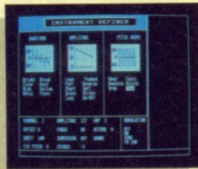
Instrument definer allows you to define your own instrument pitch, amplitude and wave forms
